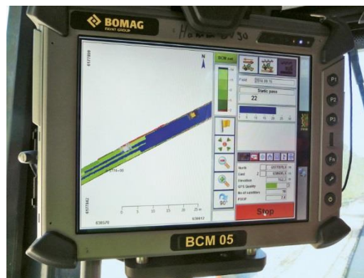
Fig. 5. Tablet-PC showing a “compaction-map”
