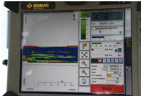
Fig. 11. Tablet-PC displays the No. of dynamic passes
