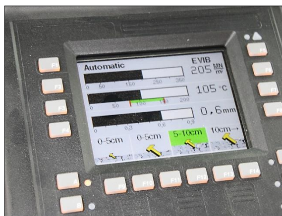
Fig. 10. AM2 provides valuable compaction data
