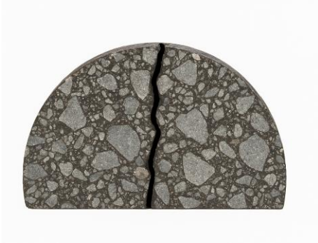
Semi-Circular Bending Test
